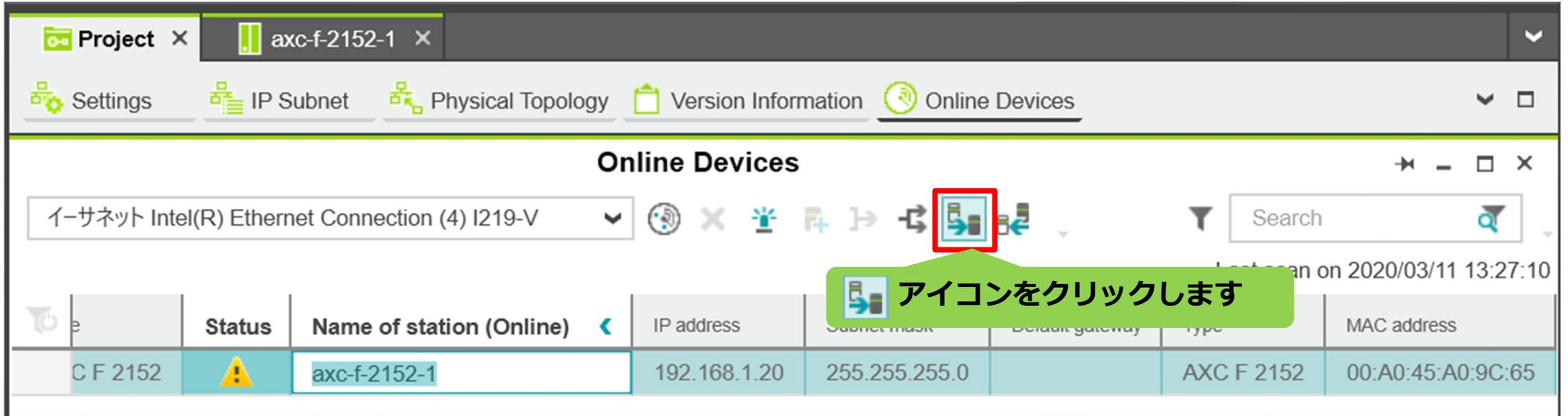
The screenshot displays the 'Online Devices' window in the PLCnext Control software. The window title is 'Online Devices' and it shows a list of connected devices. A red box highlights a specific icon in the toolbar, and a green callout box with the text 'アイコンをクリックします' (Click the icon) points to it. The table below shows the device 'axc-f-2152-1' with IP address 192.168.1.20.
